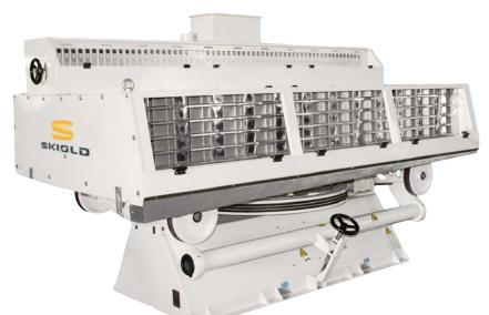
The SB table makes a sharp separation of the material into 2 fractions - usually a light on and a heavy one. Unlike other systems, the SB table is also capable of separating materials with the same gravity, but with different bouncing effect.
